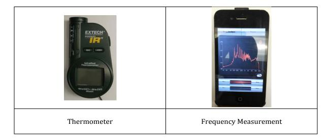
For **temperature** measurements, I used an infrared thermometer. You point it at the tuning fork and press a button and the temperature read out. This has an accuracy of one degree. It is an *Extech* Pocket IR model IR201 laser pointer thermometer.
