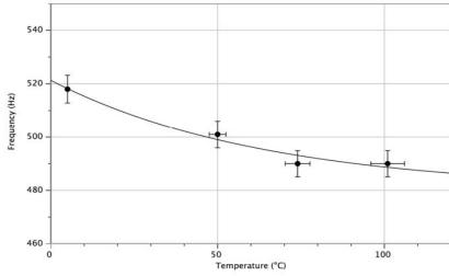
For the uncertainties in frequency and temperature I simple adjusted the percentage number in LoggerPro so that the best-fit graph line would include all the data ranges. This was as low as 1% for the frequency and 5% for the temperature; both of these are good for my experiment.
