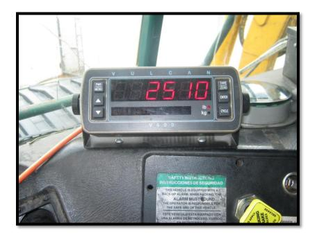
Recyclables are weighed at each location using On-Board vehicle scale. Scale reads 2,510 pounds.
