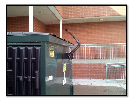
Gravity locking bar after dumpster has been emptied. Notice lock is still there! The gravity locking bar needs to be manually pushed back to the locked position. Please push the bar forward.
