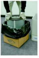
Carefully remove the filter and dispose in a plastic trash bag.
