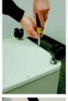
Using a Phillips screwdriver, remove the four retaining screws from the bottom cover.
