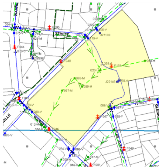
Water and Sewer As-Builts – (Courtesy of WSSC)
