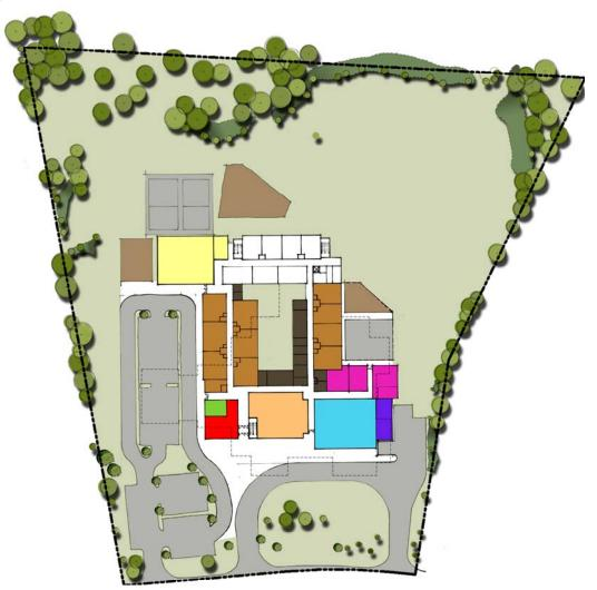
9. Scheme D is a 2 story U-shape scheme which has a similar layout to Scheme B. Public spaces are on ----
