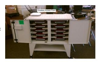
Carts must be plugged into both power and an Ethernet drop to work. Charging function and WAP (wireless access point) need power to function. If there is an issue, make sure the surge protector is turned on. All carts have wheels for movement around the building and between rooms.
