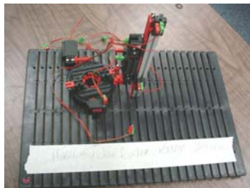
An operable Fischertechnik project which simulates a drill press in a manufacturing process.
